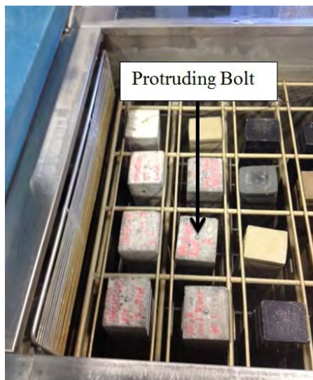
c) Freezing and Thawing Test Machine
