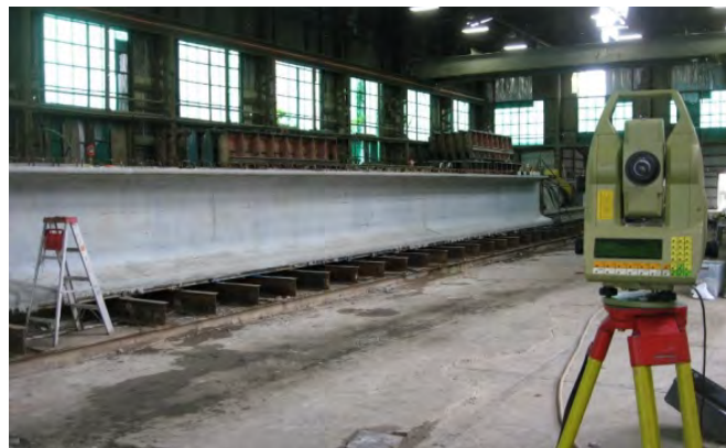
Figure 4-8. Total Station (Leica TCA2003)
