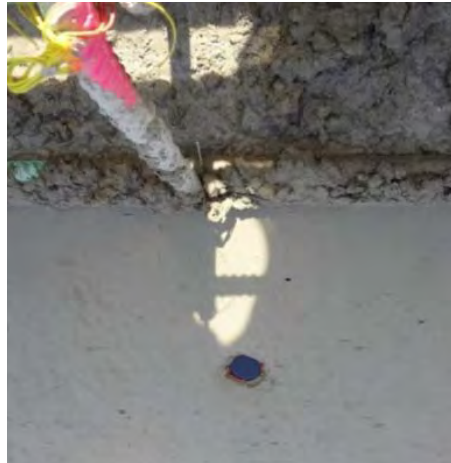
Figure 5-66. RFID Corrosion Sensor Embedded within CIP Deck
