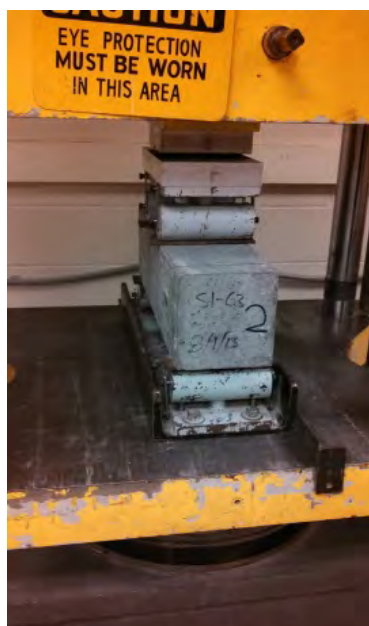
Figure 3-6. Modulus of Rupture Test Set Up
