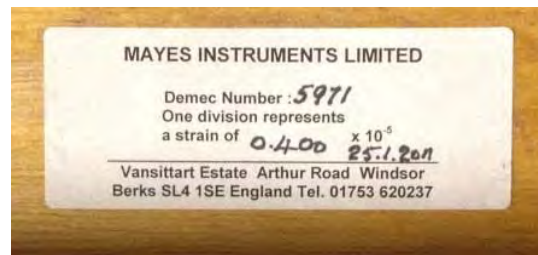
Figure 4-7. Gauge Factor Used for Shrinkage and Creep Calculations
