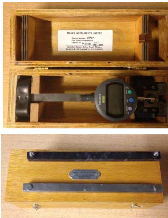
Figure 4-6. The DEMEC Gauge and Reference Bar
