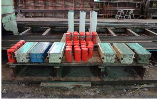
Figure 5-53. PC/PS Girders QC/QA Specimens
