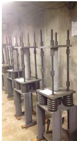
a) Creep Frames in High Bay Laboratory b) Creep Cylinder Loaded in Creep Frame
