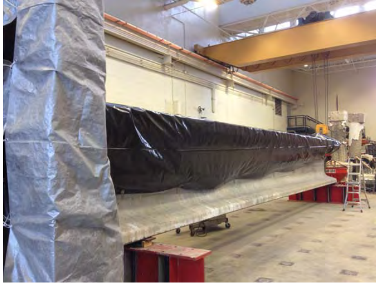
Figure 5-21. Tarping of CIP Deck
