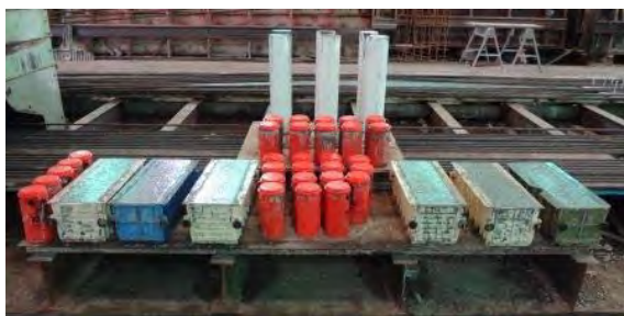
a) Precast Girder QC/QA Specimens
