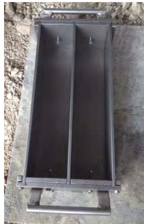
Figure 3-11. Freezing and Thawing Specimen Molds
