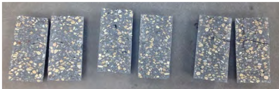
Figure 6-3. Splitting Tensile Strength Failure Plane
