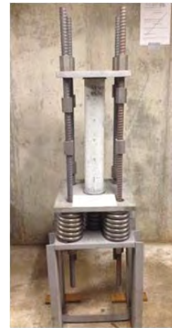
a) Creep Frames in High Bay Laboratory b) Creep Cylinder Loaded in Creep Frame
