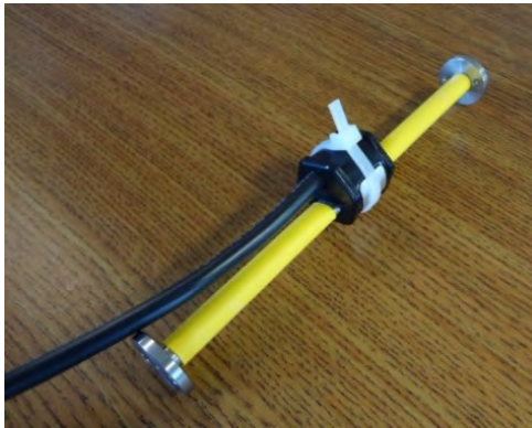
a) VWSG Secured with Zip Tie
