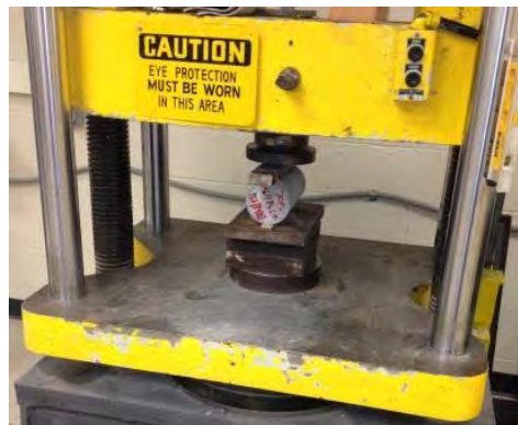
Figure 3-5. Typical Splitting Tensile Test Set Up
