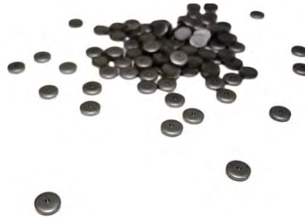
Figure 5-44. Stainless Steel DEMEC points
