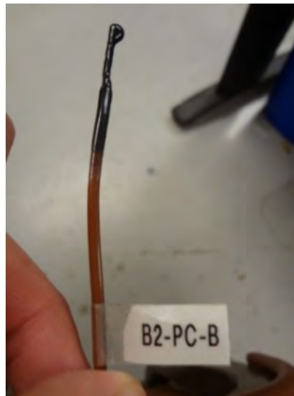
Figure 5-32. Thermocouple Preparation Prior to Field Installation
