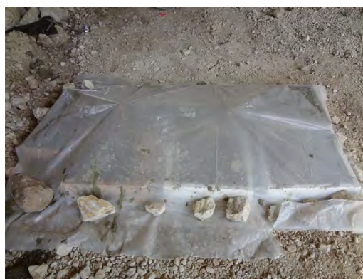
c) Curing Freeze-Thaw, Abrasion and Ponding Test Specimens
