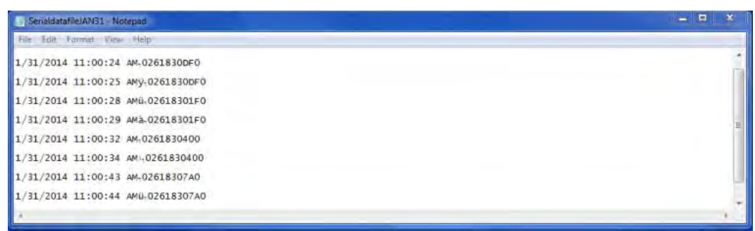
Figure 4-18. RFID Sensor’s Output File
