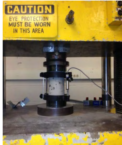
Figure 3-4. MOE Test Set Up
