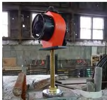
Figure 4-9. Reflecting Prisms Mounted on PC/PS Girders (Precast Plant)
